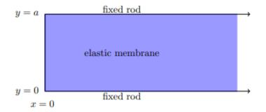
It is attached to fixed rods along y = 0, z = 0 and y = a, z = 0 from x = 0 to  $\infty$ .  $\psi(x, y, t)$  is the z displacement of the point on the membrane with equilibrium position (x, y, 0). For small oscillations,  $\psi$  satisfies the two-dimensional wave equation,
