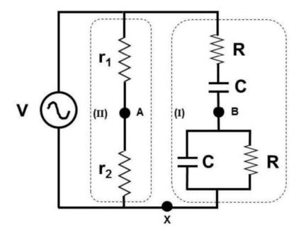
The circuit above is called a Wien bridge, frequently used in RC oscillators, and consists of two branches (I) and (II) that are enclosed by dashed lines. The voltage source produces an AC voltage with amplitude V and angular frequency ω. Express your answers below in terms of these and other constants given in the diagram.
