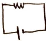
Battery spends energy and energy is dissipated by the wire.
